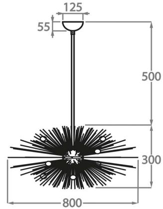
The dimensions of the central supporting chain or rod and ceiling rose are not included in the height measurements.
