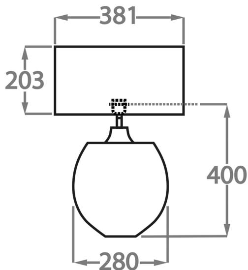
Dimensions are measured from the base of the lamp to the middle of the bulb holder and are excluding shade.
